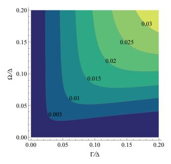
FIG. 5. (Color online) Contour plot which shows the cooling rate  $\gamma_c$  in Eq. (19) as a function of  $\Omega/\Delta$  and  $\Gamma/\Delta$ .
