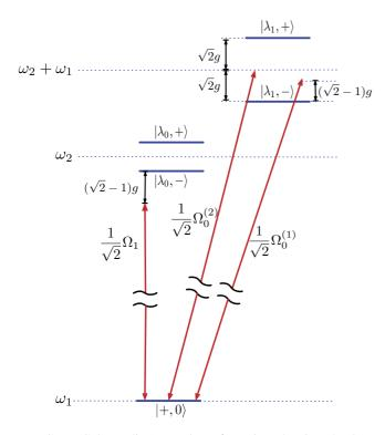
FIG. 7. (Color online) Level configuration showing the laser driving, Rabi frequencies, and detunings experienced by the target state  $|+, 0\rangle$  in the dressed state. For simplicity, we show only the least detuned couplings.
