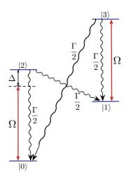
FIG. 2. (Color online) The toy-model level scheme. The 0–2 and the 1–3 transitions are driven by a laser field with Rabi frequency  $\Omega$  and a detuning  $\Delta$  with respect to the 0–2 transition. The excited atomic states both decay spontaneously into  $|0\rangle$  and  $|1\rangle$  with a decay rate  $\Gamma/2$ .
