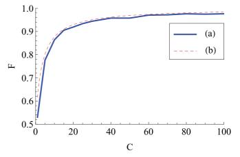
FIG. 9. (Color online) Stationary state fidelity *F* of the proposed entangling scheme for different spontaneous decay rates  $\kappa$  and  $\Gamma$  and  $\Omega = 0.03 g$  obtained from a quantum jump simulation. Here  $\kappa$  and  $\Gamma$  are varied such that the cooperativity parameter *C* remains constant at C = 25.
