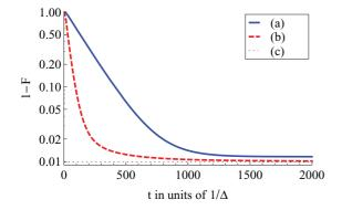
FIG. 6. (Color online) (a) Logarithmic plot of the time dependence of the distance 1 - F from the target state  $|0\rangle$  for the case where the system is initially in  $|1\rangle$  and where  $\Gamma = 0.2 \Delta$  and  $\Omega = 0.05 \Delta$ . (b) Same as (a) but for a time-dependent laser pulse with a Rabi frequency  $\Omega(t)$  as in Eq. (22) with  $\Omega_0 = 0.05 \Delta$ . (c) Theoretical minimum for 1 - F obtained from Eq. (23) for  $\Gamma = 0.2 \Delta$ .
