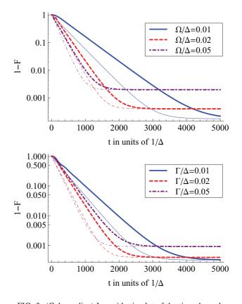
FIG. 3. (Color online) Logarithmic plot of the time dependence of the distance 1 - F from the target state  $|0\rangle$  for different values of  $\Omega/\Delta$  and  $\Gamma/\Delta$ . The system is initially in  $|1\rangle$ . In the upper plot we have  $\Gamma = 0.2 \Delta$ . In the lower plot we have  $\Omega = 0.05 \Delta$ . The thick lines are the numerical solutions of the rate equations in Eq. (10). The thin lines illustrate the analytical solution in Eq. (21).
